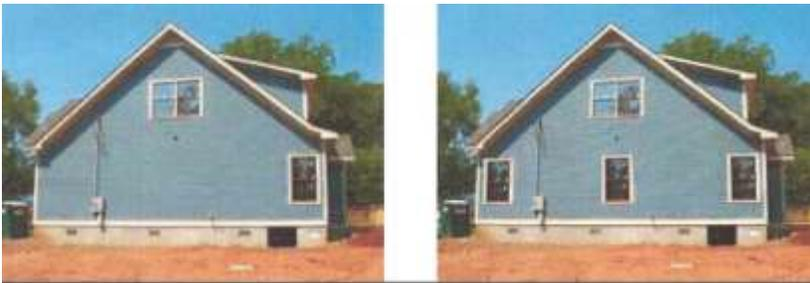
The image on the left shows a side elevation with a large expanse of wall without windows or other details. The image on the right shows the same elevation if several additional windows were added.
